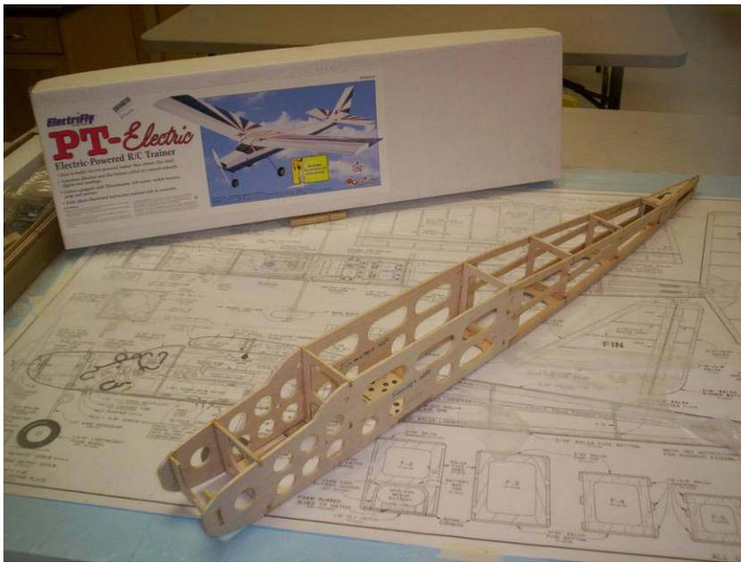
The PT Electric kit by Great Planes was chosen as our first R/C construction project. (Pic-7) It is a 56" wing span trainer with an old style brushed motor. The kit uses a switch and a servo to turn the motor on or off. No ESC. The kit has elevator and rudder only. Some consideration was given to adding ailerons but this being our first kit we will be sticking with 3 channels. The only modification to the plan will be to use a brushed ESC on the stock motor and a larger battery.
